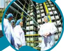
Production and package area of packed milk and automatic system transferring finished goods from production area to intelligent warehouse.
