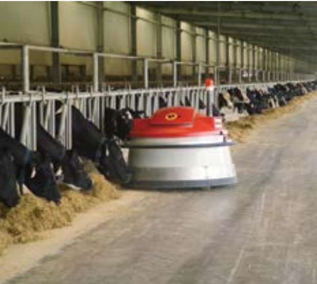
Automatic feed pushing robot
